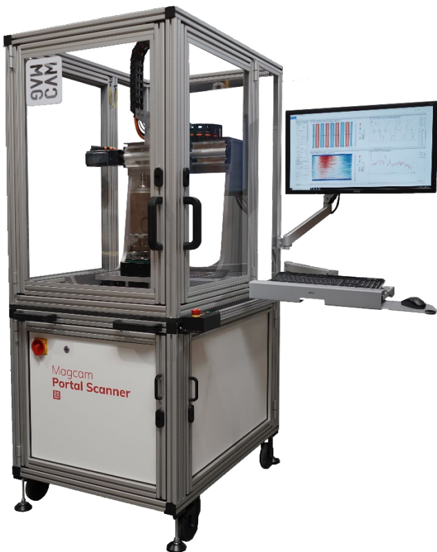
Left: Magcam Combi Scanner with 300mm x 300mm x 300mm scan range in a safety housing. Right: Automatically recorded and stitched magnetic field images of a large magnet.
